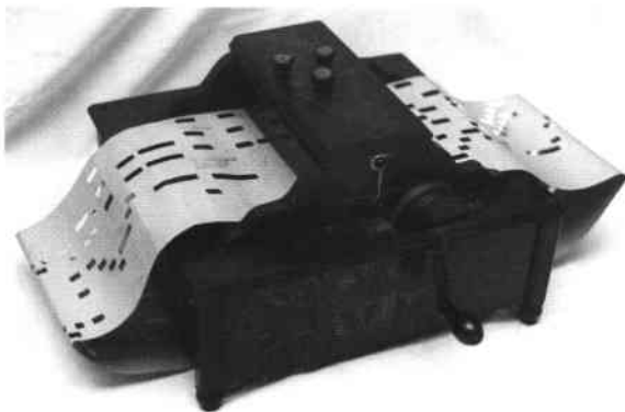
Fig.4 The "Orchestral Organette", the subject of J. M. Draper's 1887 patent, this particular example being very close to the patent drawings. (see Part 2). The three stops are: 'Flute', 'Vox Humana', and 'Expression'. The reeds for the 'Flute' are tuned as in the "Victoria" and "English", those for the 'Vox Humana' are an octave higher but tuned slightly out of key to give a 'beat'. The "Expression" stop partially covers both sets of reed openings with flaps to reduce the volume of sound.
