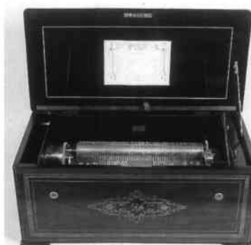
Fig 2. Flute Voix Celeste box by B A Bremond. The seventeen key reed organ section can be seen in the centre of the cylinder.
