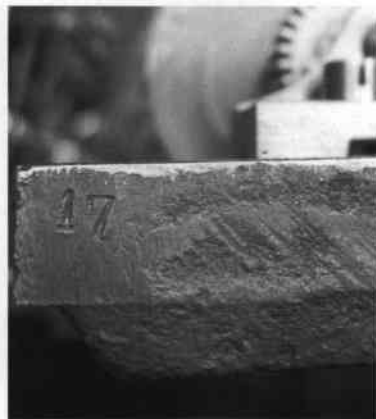
Fig. 11. Blank 17 on bass edge of bedplate. The casting is strengthened with a rib below, as is also visible in Fig. 10.
