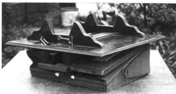
Fig.5 The Orchestral shown in Fig. 4 but with bottom framework removed to show the two exhausters and reservoir. It can be clearly seen here how the reed block assembly fits into a flat bottomed 'V' and is held there by two hooks.
