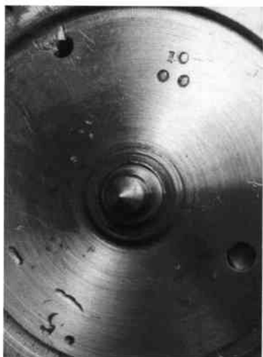
Fig. 3. The great wheel is also stamped blank no. 5 for the cylinder assembly.
