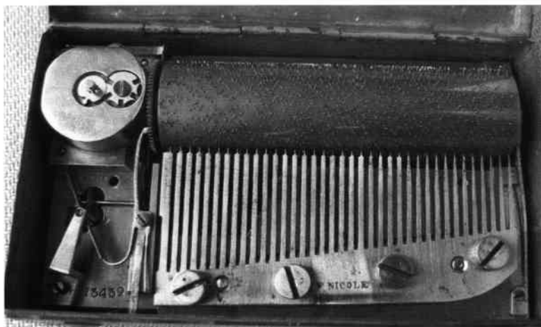
Fig. 12. Frères Nicole 13432 made in 1833. Cylinder diameter \frac{3}{4} " (19mm), 37-tooth comb, twelve airs. Complete programme lasts 7 minutes.
