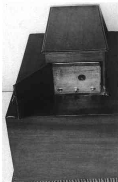
Fig. 10. Side door of the top box opened for access to controls. Plenty of headroom inside, and the musical box lid can be opened – if its side-hook is disengaged.
