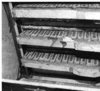
Fig 8. The reed bank. Note that each of the three banks carries pairs of reeds, one on top and the other underneath.
