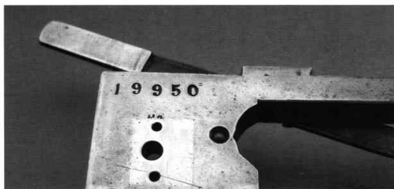
Fig. 10. Brass-tipped end for the control lever. Polished top of bedplate leg visible in screwed hole, countersunk for stylish finish. (Another is at top right of Fig. 9.)
