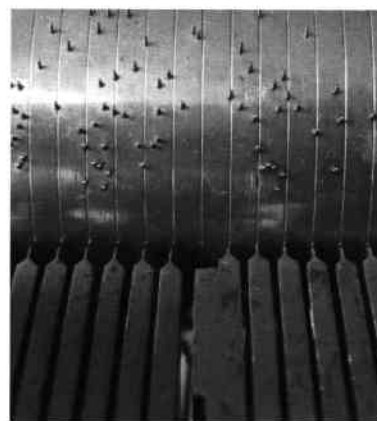
Fig. 4. Unpinned track between the bell teeth and the fat bass tooth.
