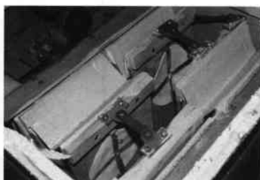
Fig 6. View of the feeders. Note the circular valves and the valve-actuating rod driving 4 feeders linked in pairs.
