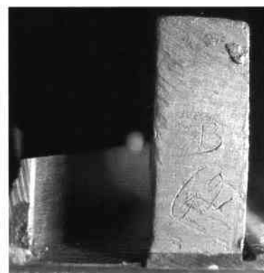
Fig. 3. The bass lead of serial 326, scribed with the cylinder blank number.
