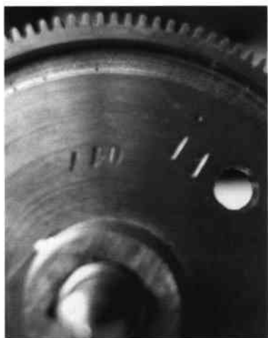
Fig. 4. Gamme 110 and blank 11 on the great wheel of serial 1112. You'd have thought sharp focus for both these side-by-side numbers was an obvious essential, but oh, no, my know-all digital camera decided to favour 11. So here it is for all to see.
