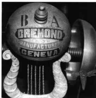
Fig. 7. A 5-string golden lyre supporting the six-bell gantry on Bremond serial 13,446 - mandolin and bells with a 15" cylinder, very nice.
