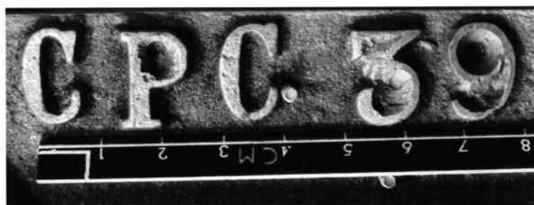
Fig. 6. Paillard's casting mark on serial 31747 bedplate. That 39 is probably the pattern number. Photo by George Worswick back in 1996 when he was helping with data for Oddments 72 and 76.
