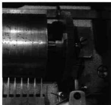
Fig. 1. The cylinder peg is resting on the highest step of the snail cam, which advances one step when its teeth engage with the finger of the tune change lever, -seen at the top.
