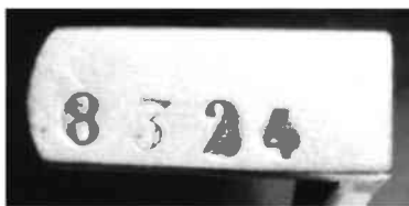
Fig. 2. Bremond number on winding lever.
