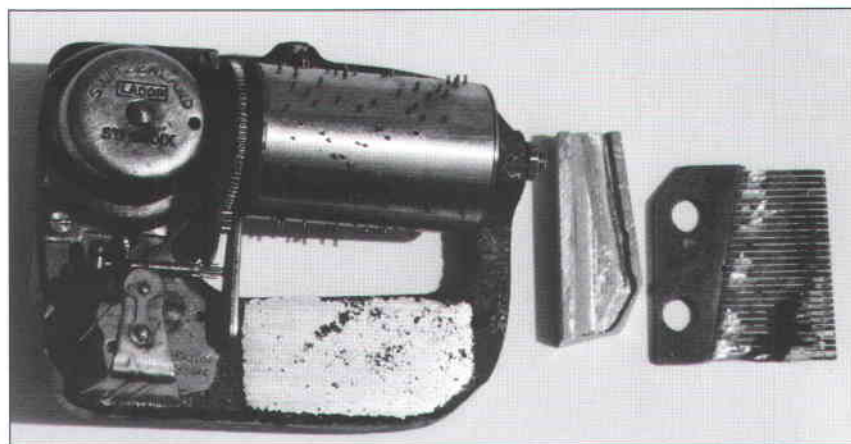
Fig 1. The re-tuned comb (right) and the comb base (centre), cut from a car door handle. The base is viewed from its underside. The thickness of the comb base is angled (about 7 degrees) such that the comb's teeth point towards the axis of the cylinder.
