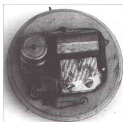
Figs. 2, 3 & 4: These are restorations comprising reproduced parts and original parts. The original cylinders were stripped and replaced with the ones shown, the programmes being exact copies of originals.
