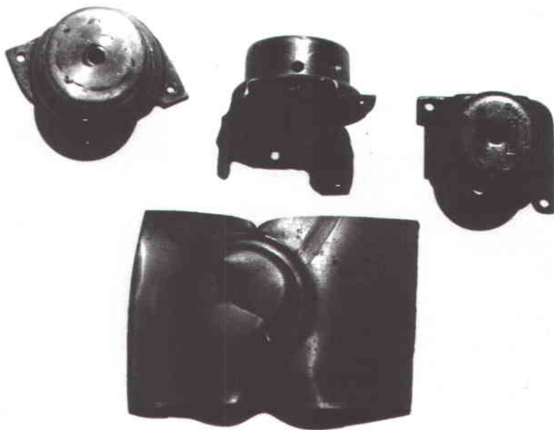
Fig. 7: An original Lador case (right) with a failed attempt to deep draw a replica. Top left and centre are fabricated replica cases. The left one has yet to be skimmed and polished, the centre one shows the cylinder bearing and indented spring retaining lug
