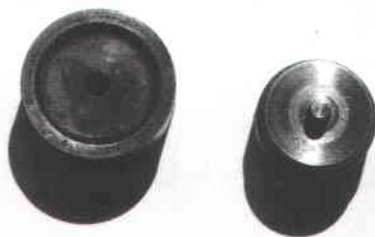
Fig. 7: A press for final shaping of a crown wheel. The male part has a fixed spigot to hold the blank central to the die.
