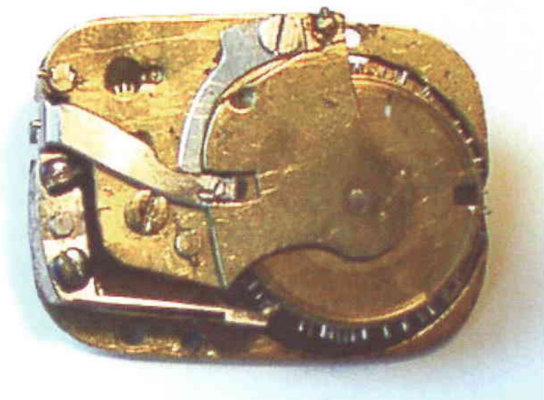
Fig 2. A barrillet movement, showing the pinned mainspring barrel (right) and the comb, bottom left, seen on edge.
