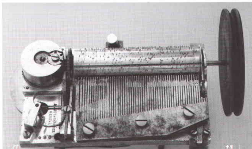
Fig. 6. Typical petite musique serial 480, with drive as often found in rocking ship automata.
