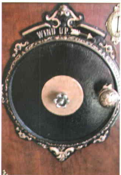
Fig 7 (left). Roepke winding handle showing fixing nut.
