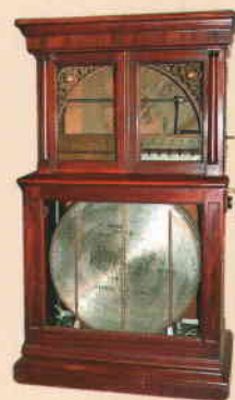
»Regina Changer Mod. 33, c. 1900« Largest automatic changing model for 12 metal discs (27 in.)
