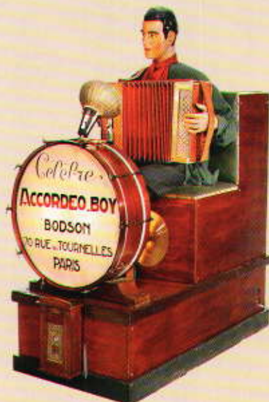
»French Automatic Accordeon Player "Tino", 1925« A lifesize accordeon boy with moving head, eyes, lips and eyebrows; pneumatic paper roll operated system. – Perfectly working!
