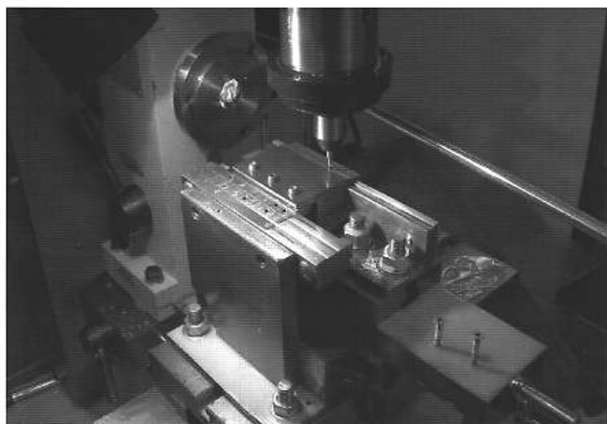
Fig 6 Segment with tip and damper slots being milled
