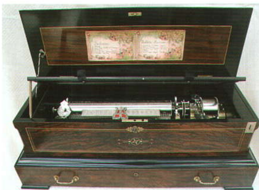
Seen and heard at the MBSGB Spring meeting, a 6-air interchangeable box by Mermod Frères, coin operated and with two cylinders, recently restored in Switzerland by Musée Baud.
