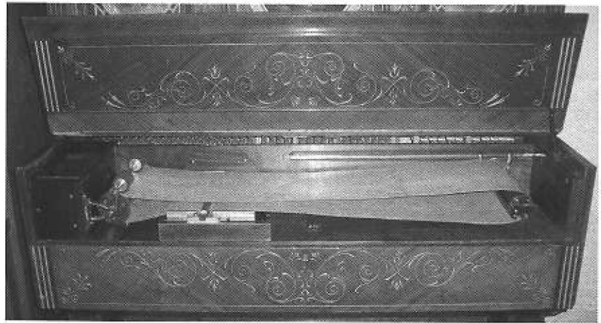
Fig 2. The Player Shelf with endless band
