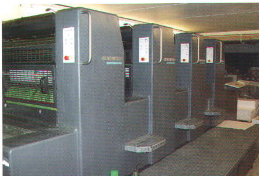
3. The four parts of the press are clearly shown here; this machine would cost over £750,000 if new today; it is kept running for 15 hours a day whenever possible.
