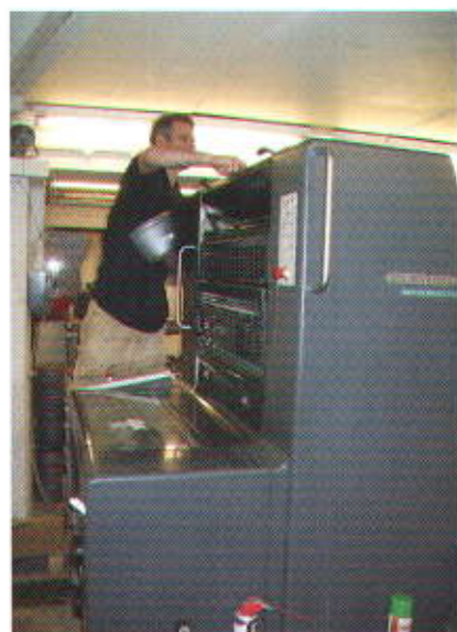
2. Putting more Yellow ink into the printing press.
