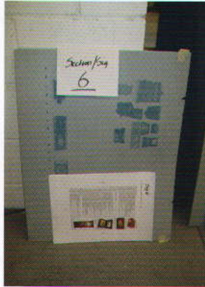
1. A set of printing plates for one of the sections of the book; notice this is for one of the 'colours' so does not have any text.
