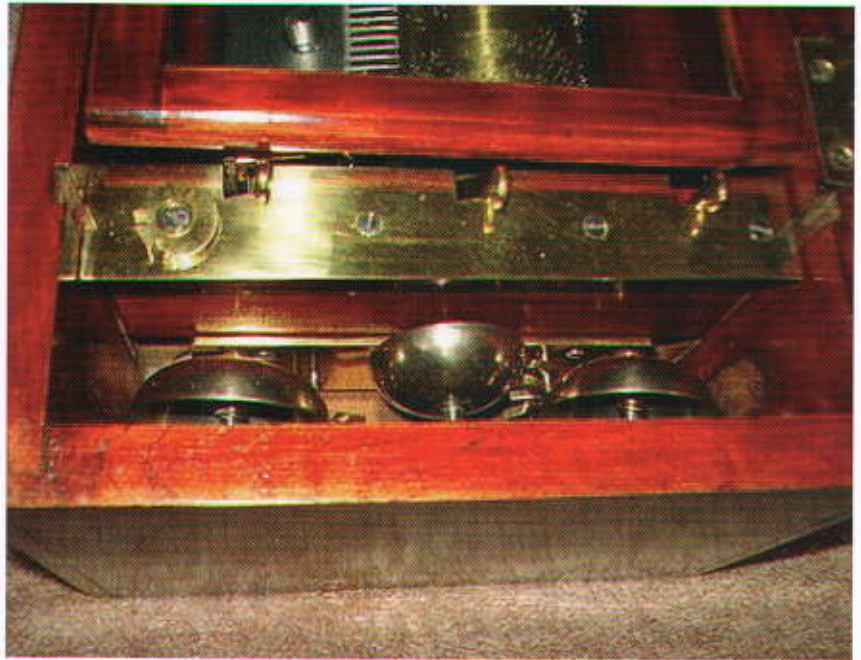
Serial 26250, showing the three bells and control levers. The Geneva stop is apparently mounted there to stop it from getting lost!
