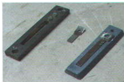
Frame with sloping sides on which the new reed is riveted (r.h.) left: a classic reed frame from which the replacement reed was taken. Centre: the old broken reed
