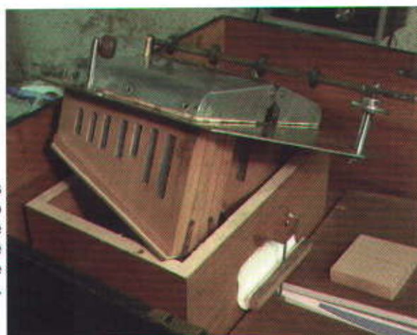
The reassembled musical mechanism ready to be replaced in its housing. The two tinplate caps which go over the reader rise up to create a 'forte' effect. Their edges are sheathed with a white leather which prevents a metallic noise when they return to the 'piano' position. At the front of the housing, the curtain for the exhaust.
