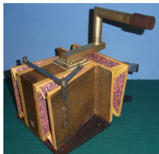
Fig 5 The pump is a wooden box on each side of which are hinged wooden bellows plates
