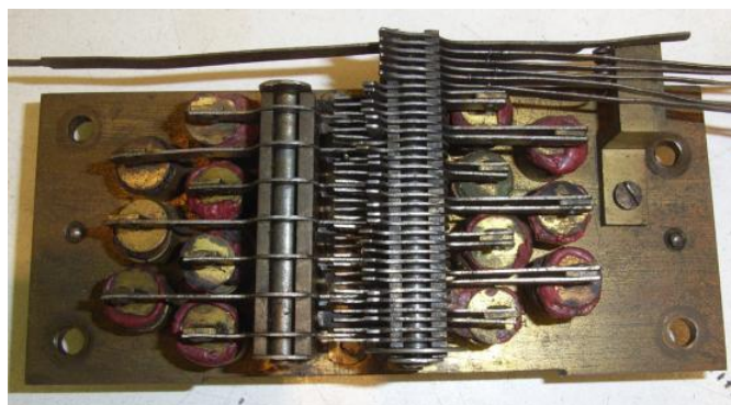
Fig 7 The gantry repaired with blobs of sealing wax to hold the pallet leathers in place
