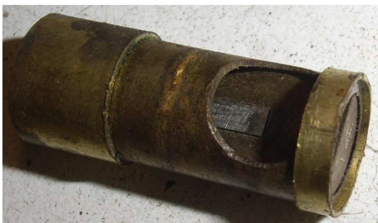
Fig 4 The reeds are each held in a small brass tube
