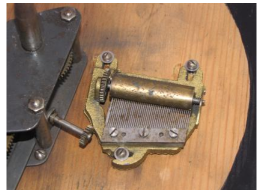
Fig 3 Device for turning the music on & off
