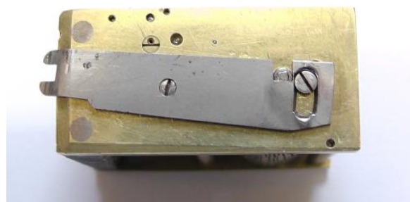
Fig 11 The tune-change lever
