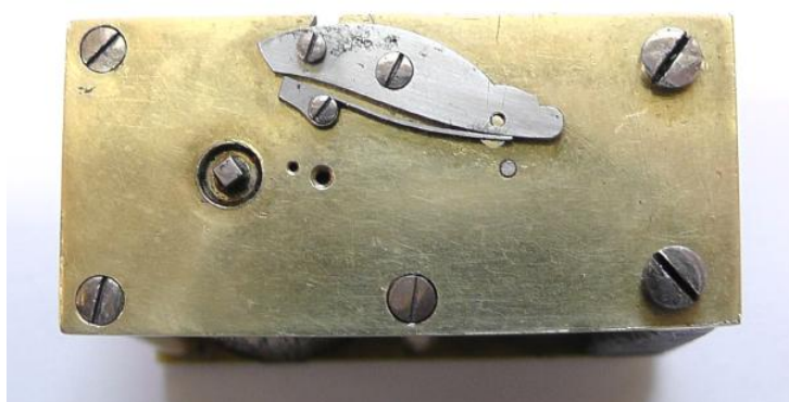
Fig 9 The start/stop lever
