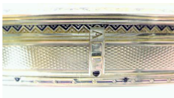
Figure 10 The tune-change slide
