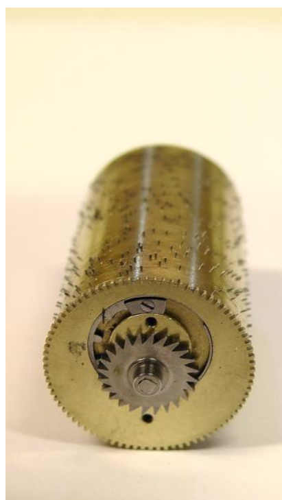
Fig 4 The cylinder with its ratchet wheel
