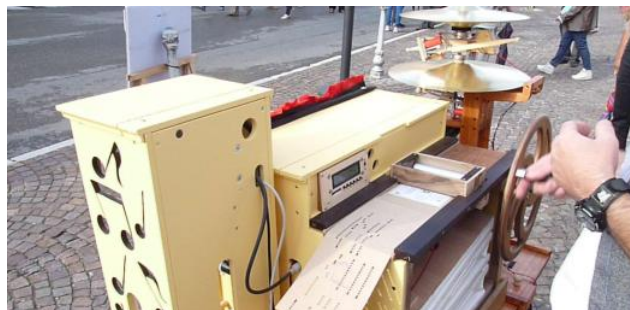
Flavio's instrument is programmed by a punched card book
