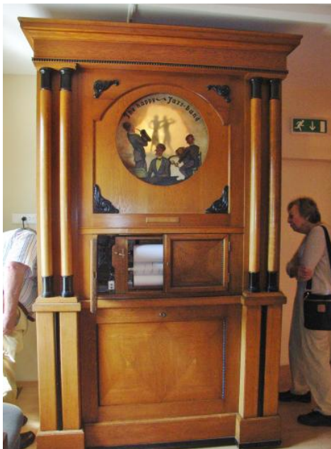
Poppers Jazz Band Orchestrion, made around 1925 in Leipzig. This is a pneumatic roll playing piano orchestrion, with percussion on the top, having one large and one small drum, a cymbal, a wood block and a triangle. The piano itself has a Mandolin rail.
