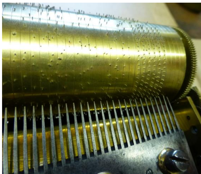
Fig 2 The movement is pinned for repeat notes at the treble end
