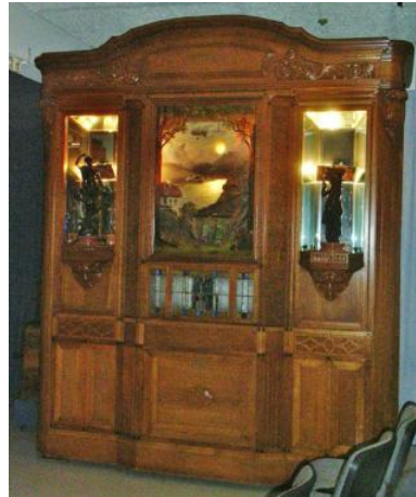
A Hupfeld Helios Piano Orchestrion model II /26, one of only two recorded. (This is almost guaranteed to uncover another). Made around 1920 in Leipzig, it has various pipe ranks, which could be ordered from choice, and various volumes, done by altering and re-voicing the pipes. As the roll is playing, behind the front there are moving pictures.
