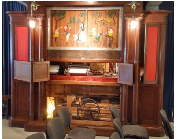
A Weber Maestro made around 1925 by Weber and Co of Waldkirch. There are ten different instruments in the cabinet, namely piano, mandolin, violin, trumpet, clarinet, flute pipes, xylophone, tambourine, cymbal and snare drum. This also has a gramophone fitted on the right-hand side, one of only eight known. It plays from specially arranged 88-note rolls.
