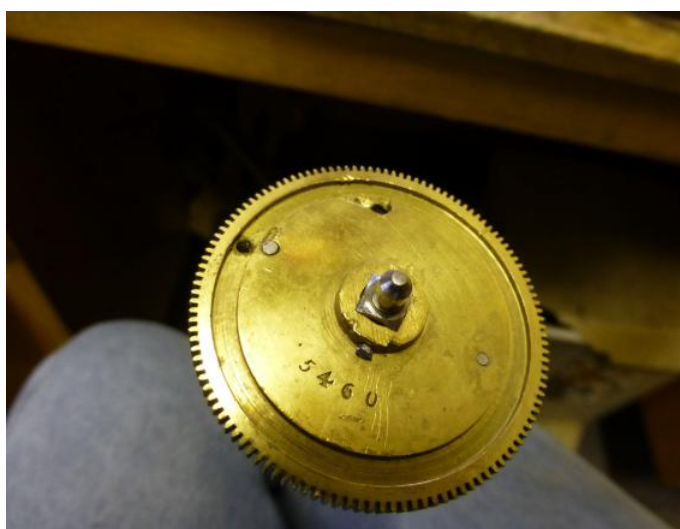
Fig 4 There is a tapped hole in the middle of the stop/start track on the great wheel
