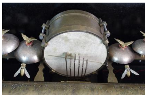
The drum of the Troll box showing a wire across the drum to use as a snare
