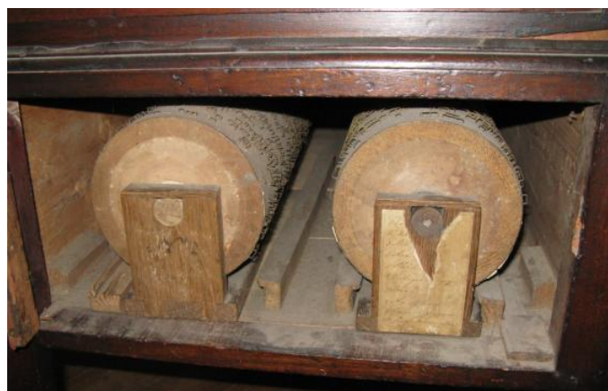
Barrels 2 and 5 (on the right with a damaged tune sheet on the end of the barrel carrier), housed in a cabinet under organ
