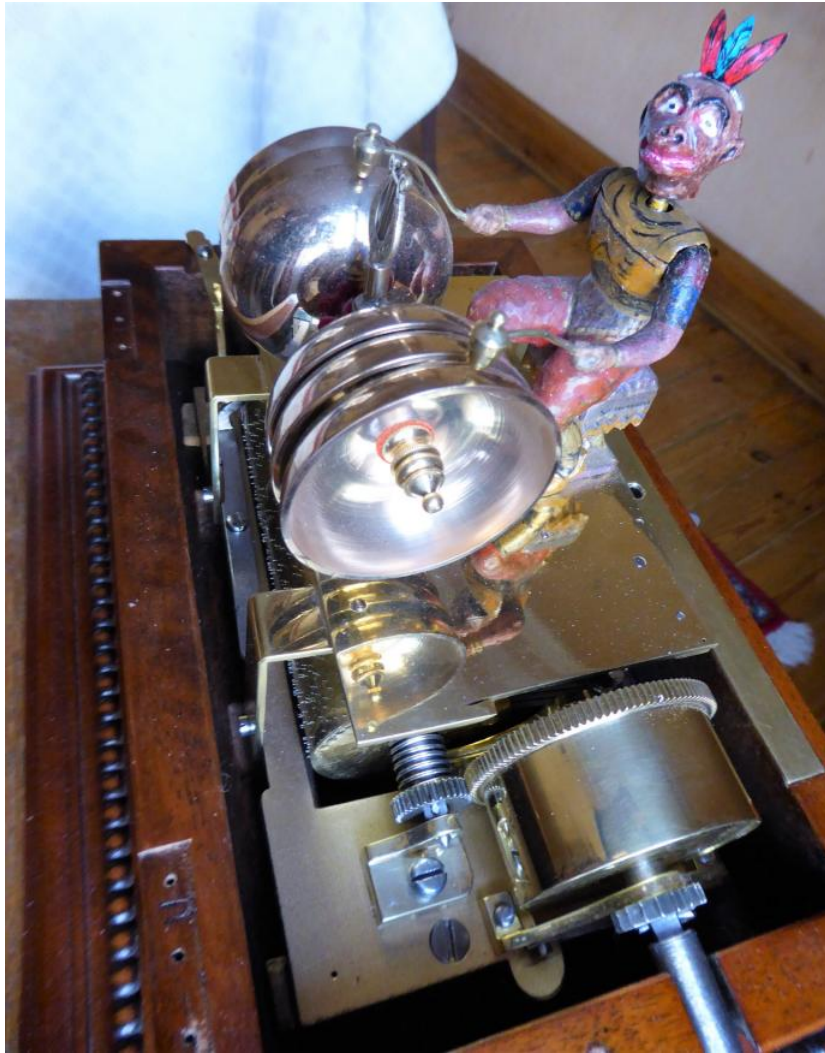
Fig 6 Cylinder great wheel of the movement. In its centre there is screwed a disc a few millimetres thick which has a cut-out profile on its horizontal plane, and whose outer edge has steps of different height, filed in the thickness of the piece. These are the two cams, perpendicular to each other, which are necessary for the two movements of the head.
