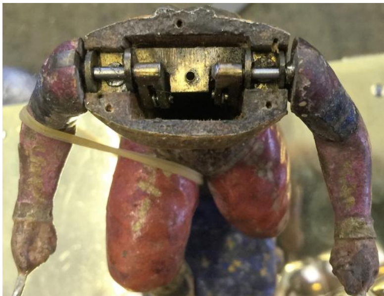
Fig 10 View of the upper part of the automaton's body. One can see the head's central 'left-right' movement tube into which the up-down movement rod slots. On either side you can see the articulations of the automaton's arms.
