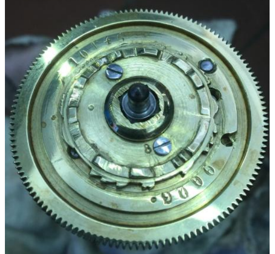
Fig 6 Cylinder great wheel of the movement. In its centre there is screwed a disc a few millimetres thick which has a cut-out profile on its horizontal plane, and whose outer edge has steps of different height, filed in the thickness of the piece. These are the two cams, perpendicular to each other, which are necessary for the two movements of the head.
