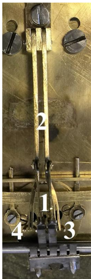
Fig 16 This view shows in part the linkage necessary for moving the arms. The rods (1) linked to the tooth at one end are fixed to their corresponding rods (2) which they raise. At the end of rod (2), which is in the shape of a fork, is fixed a third rod (3 or 4, not visible) which passes through one of the two holes cut in the wheel and which rises through the automaton's body, up to the shoulder joint. (See Fig 11.)
