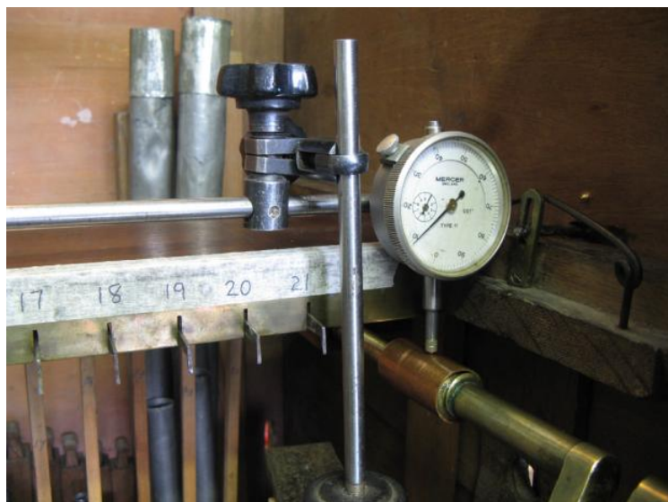
Fig 20 Clocking the runout on the bent crankshaft
