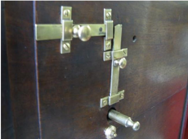
Fig 13 Barrel latching device. Horizontal bolts are pulled forward to raise the key frame, allowing a vertical knife to be raised so freeing the brass peg.
