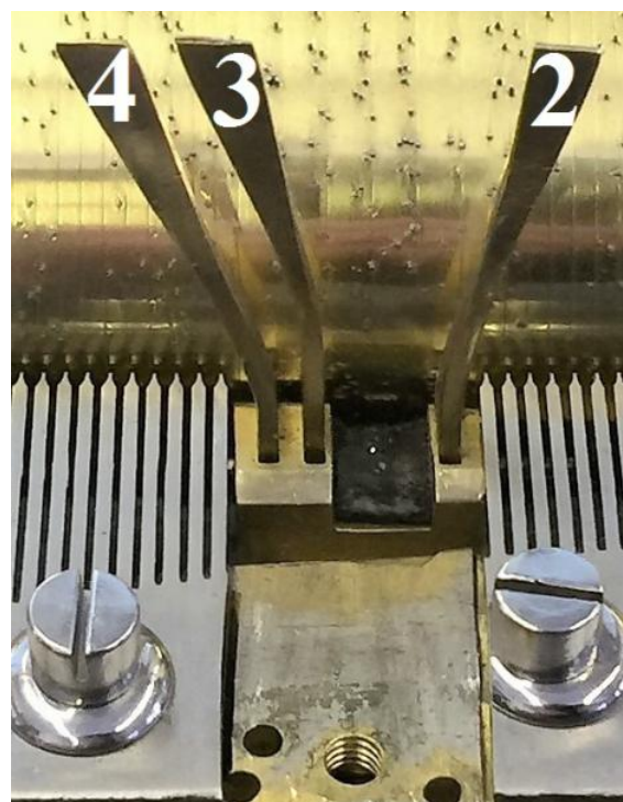
Figs 13 This and Fig 14 show the feelers 2-3-4 which by pivoting backwards when a pin passes, push the levers 2-3-4.
