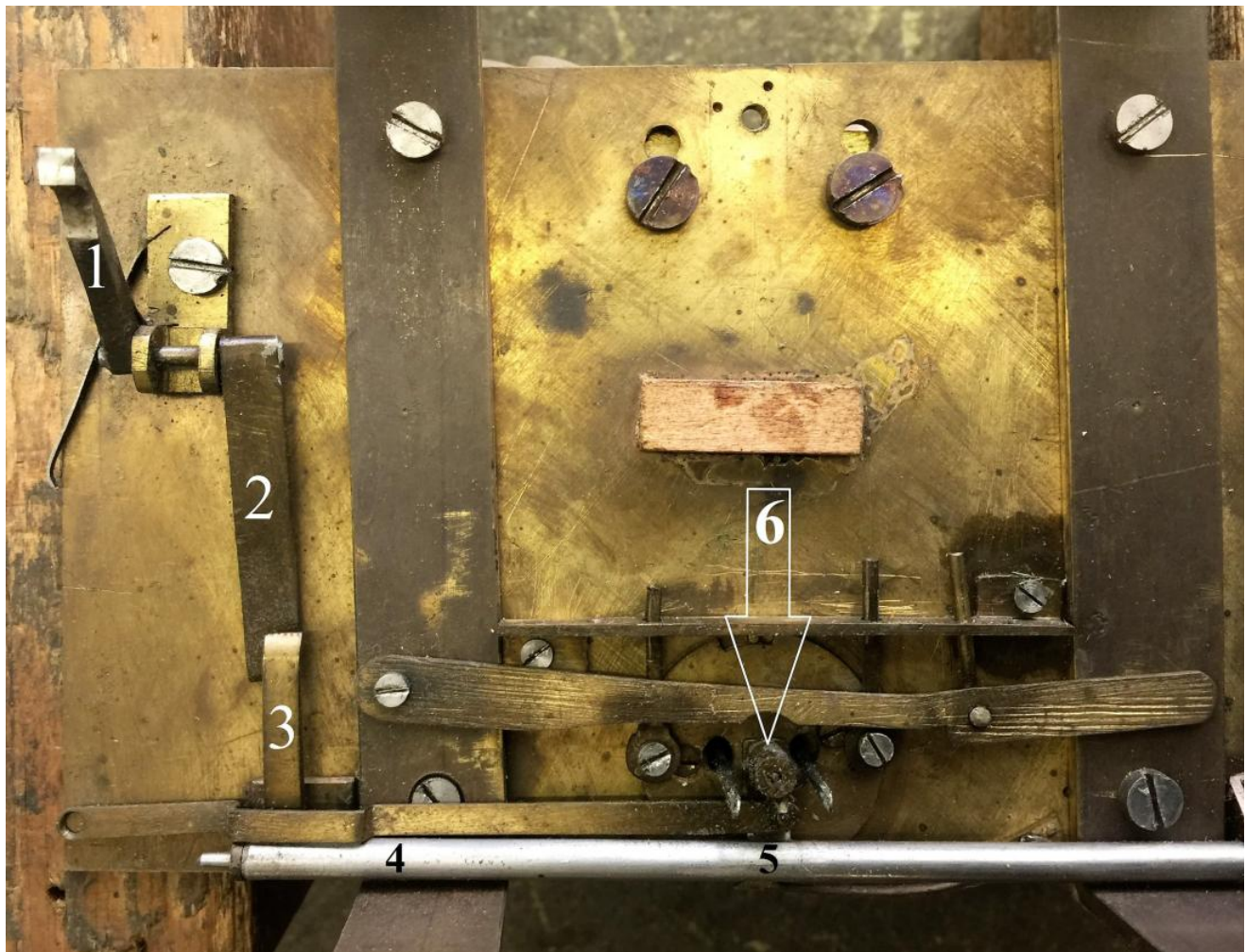
Fig 8 At top left can be seen the feeler (1) which, set upright by the cam, makes element (2) swing, which in turn causes element (3) to move. This strip (3) is fixed to the axle (4) which then rotates. At the marked position (5) on the axle is fixed another strip in the shape of a fork which pulls the cylinder marked with an arrow (6) downwards (but shown as upwards in this photo which is presented upside down). In the centre of this cylinder one makes out the end of a rod which is interlocked with it. This rod passes through the whole body of the automaton vertically towards the head, and is inserted, at its other end, into the head, which is pulled downwards by translation of movement.
