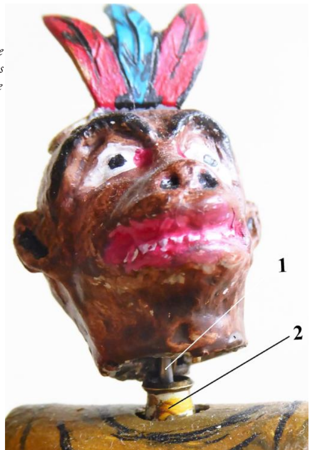
Fig 11 The back of the head is fixed to the tube (2) by a flexible link. The head, interlocked with the tube, turns. The rod (1) crosses the tube and hooks onto a little spring fixed to an armature attached inside the head which is hollow. The spring is necessary as the rod also turns. Pulled downwards, the rod lowers the head. This last movement has a smaller range than the other.
