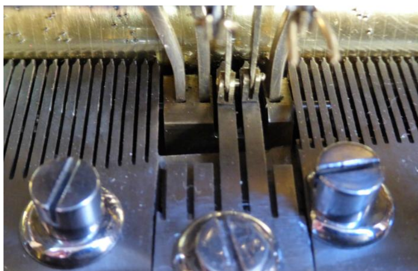
Fig 15 Inserted between the two musical combs, the little non-vibrating comb has retained only the two wide teeth necessary for each arm. Normally in bell-boxes the linkage is fixed below the tooth, while here it is above.
