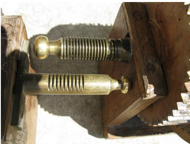
Fig 16. Barrel 1 (top) with threaded peg forming extension to barrel axis. Barrel 2 (below) with wider spaced notches on barrel carrier peg.
