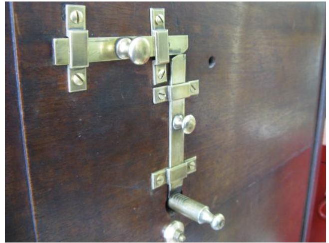
Fig 14 The knife is pushed down into the notch in the brass peg (tune six selected). The bolt is pushed back to secure the knife and the lower key frame.
