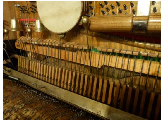
Detail showing felt-covered hammer heads on the left, and uncovered beech hammer heads on the right
