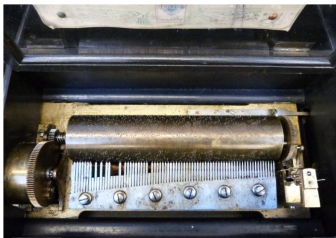
Fig 1 Silber &amp; Fleming box with damage to comb
