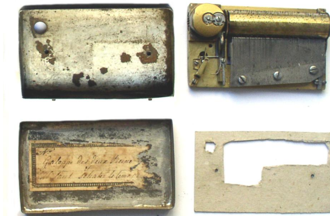
Fig 2 An early snuff box with a sheet of cardboard to prevent the pins touching the bottom of the box.
