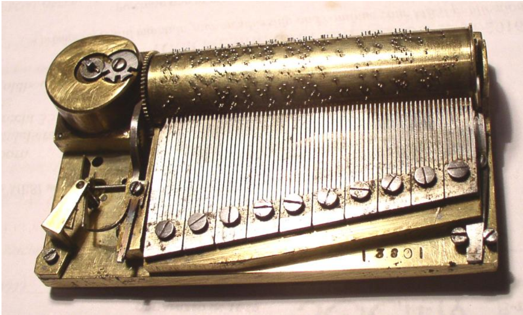
The movement of the snuff box showing ten sections each with seven teeth and the serial number 13801 impressed on the baseplate.
