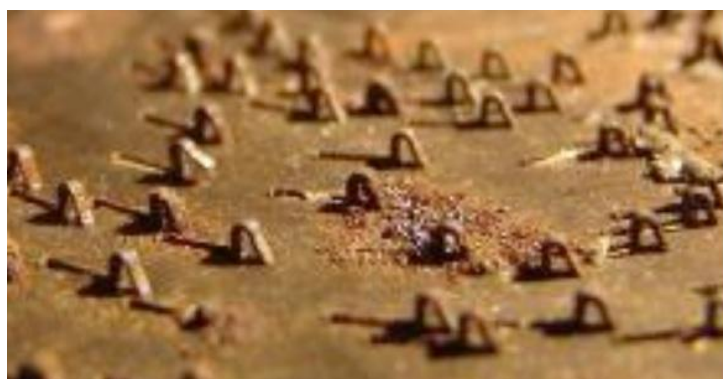
Image 4 100 year old musical disc with both surface rust and powdery corrosion
