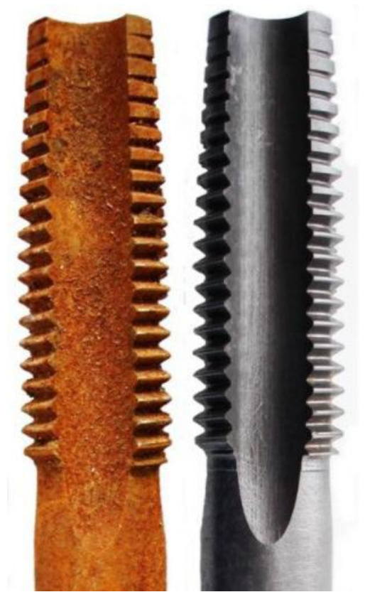
Image 9 A steel part stored in VCI remains rust free long term - versus the same part not stored in VCI packaging
