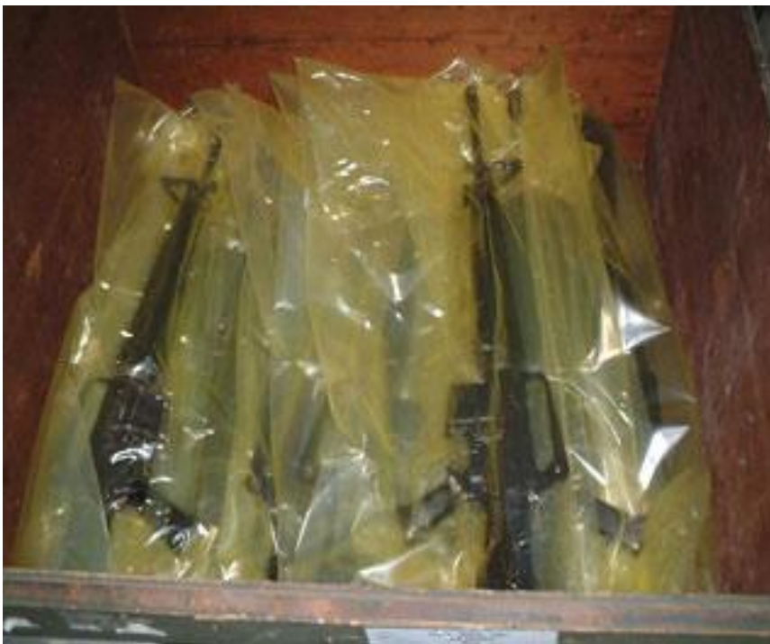
Image 10 Military forces routinely protect materiel in VCI impregnated plastic bags
