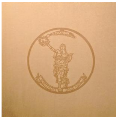
Fig 13 The de-rusted discs are then stored in this the finished disc storage folder. Bespoke from high quality kraft board, this disc sleeve contains a thickened VCI plastic bag in which the disc is easily placed and easily removed. Manufacturer information states that a VCI bag will provide around five years of continuous metal protection. In practice, they can be expected to provide at least ten years of protection (UK military working practice). 33 Note, that the VCI bag can be easily and inexpensively replaced and the same kraft board folder re-used. I have spare folders, so please contact me if you would like to order some.
