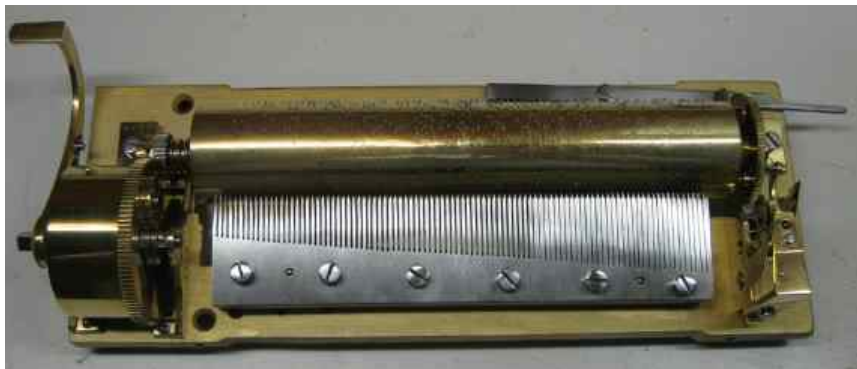
Fig 7 Swiss movement with Maly comb and cylinder
