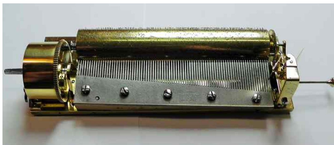
Fig 2 Swiss movement with Rzebitschek comb
