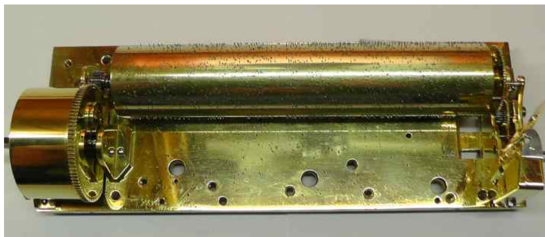
Fig 1 An early Swiss bedplate. The three large holes are for the Swiss comb screws.
