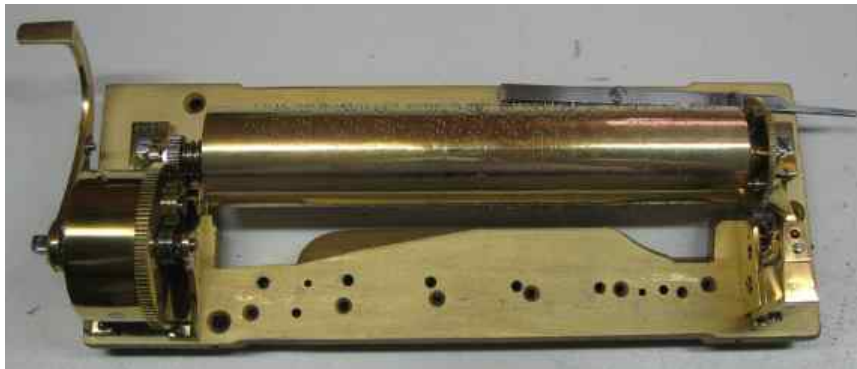
Fig 6 Cast iron Swiss bedplate with both Swiss and Czech holes, and right-hand cut-out for Czech tuning weights
