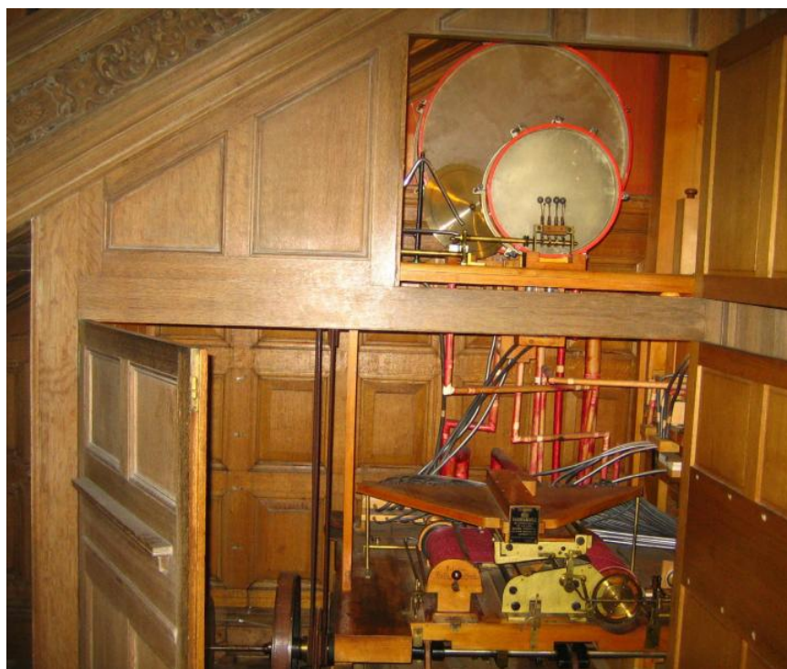
Fig 2 The pump, key, drum and roll frame situated under the stairs
