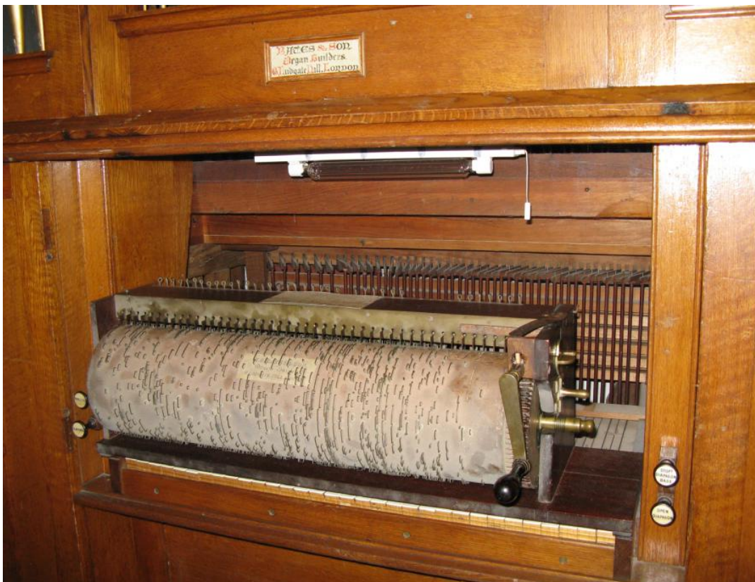
Details of the barrel. The scorch mark in the top right corner might have been from a candle set up for locating the correct tune in the darkened church.
