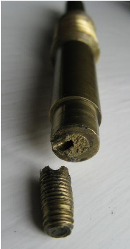
The broken end of the crankshaft
