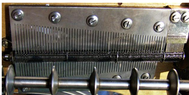
The two unequal combs and (right) the tone bar release mechanism
