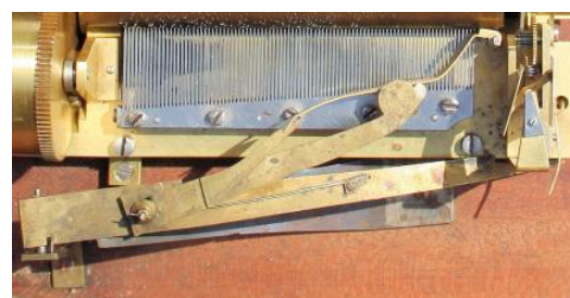
Fig 8 The movement release linkage. Exactly how this worked has yet to be determined.
