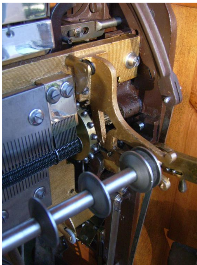
Drive wheel with sprung teeth and automatic disc-retaining bracket
