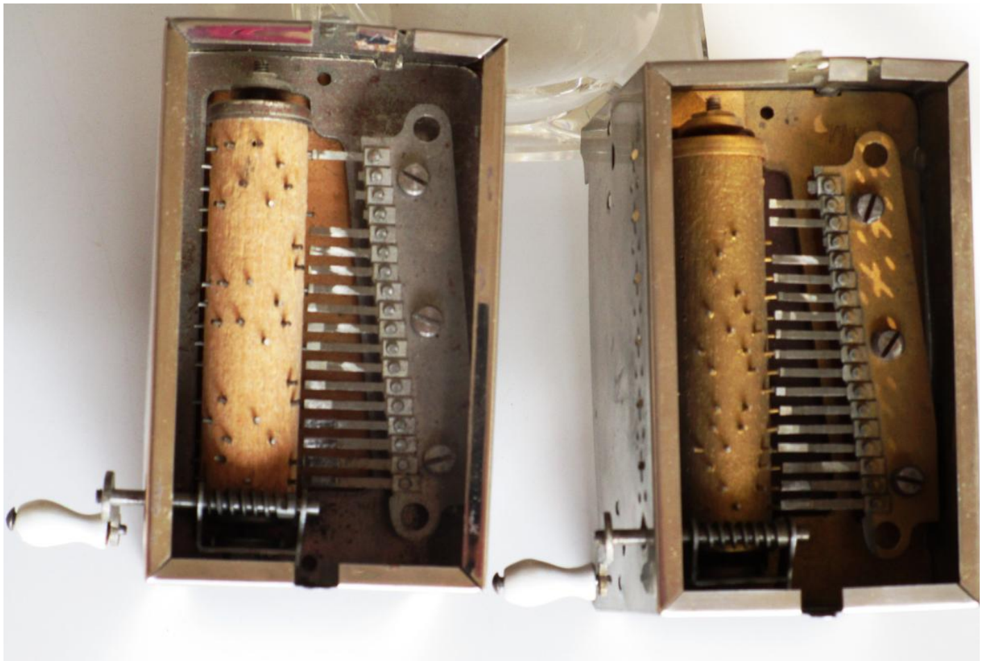
Fig 4 Two Organino movements, each with a wooden cylinder but one movement painted brass and the other not painted
