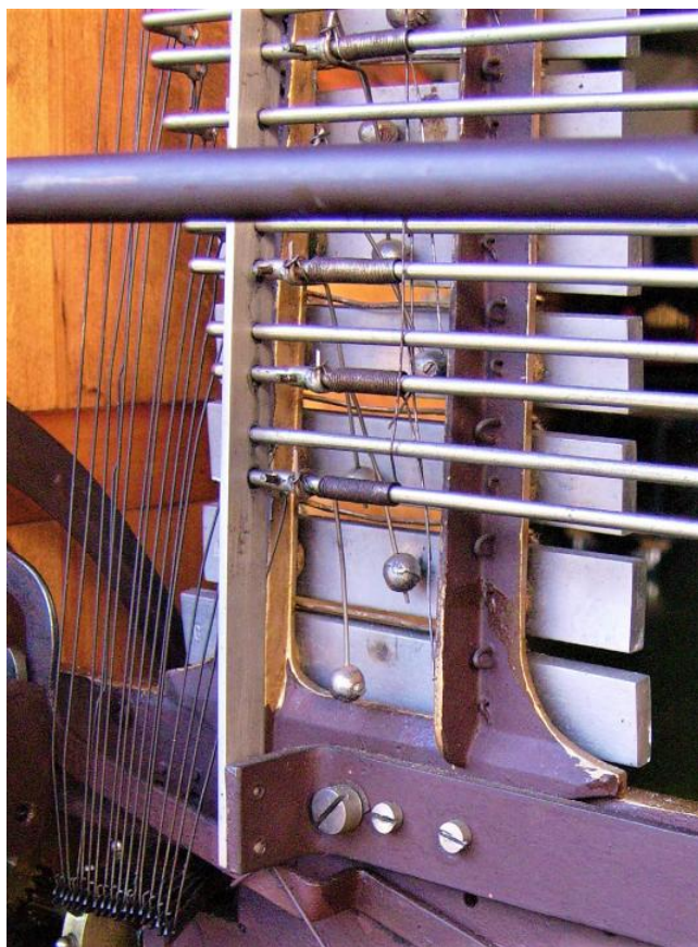
The bent tone bar weights afflicted with lead rot
