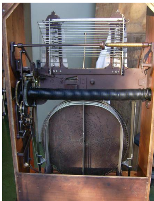
The large torsion spring with the overwound end piece (view from rear)
