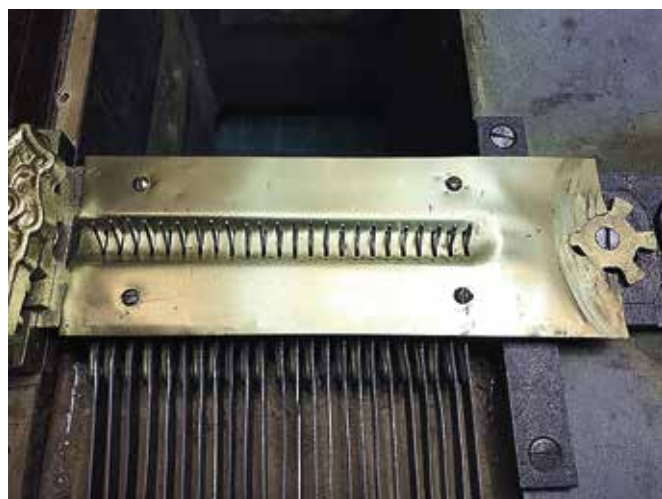
The assembled tune change mechanism showing the tune change cam wheel to the right of the 24 keys
