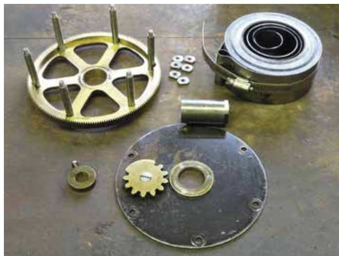
The dismantled spring motor
