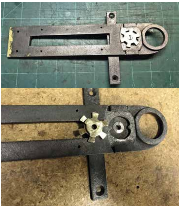
Detail of tune change cam wheel, in situ and removed
