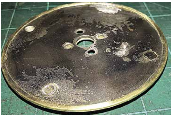
Drive disc. You can see the new pin towards the righthand side. (Note the enlarged scale of this photograph)
