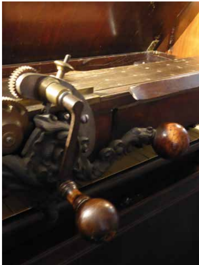
Mechanism for moving the planchettes. Note the turning handle (with knob) with ratchet lever behind, and the screw in the top of the frame holding them which is adjusted to determine which is used.
