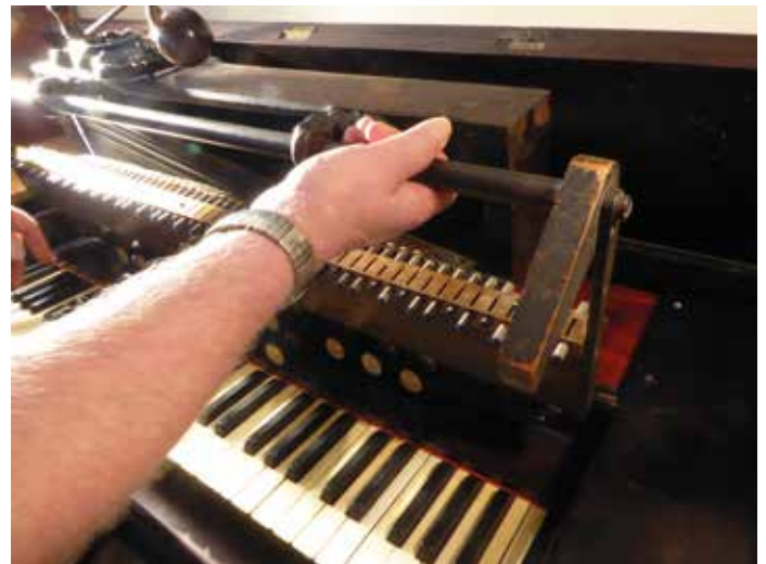
(Top) 'Rocker' mechanism being lowered into place; (Below) detail of part of 'rocker' mechanism (this example damaged.)
