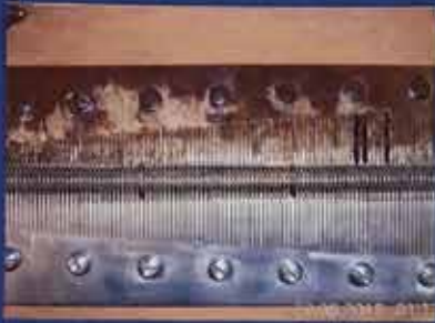
De-rusting the combs. This was done with the combs in situ on the bed plate to protect the leads. The bed was mounted on a sloping reversible wooden jig with a large slot in it to allow removal and fitting of the dampers.
