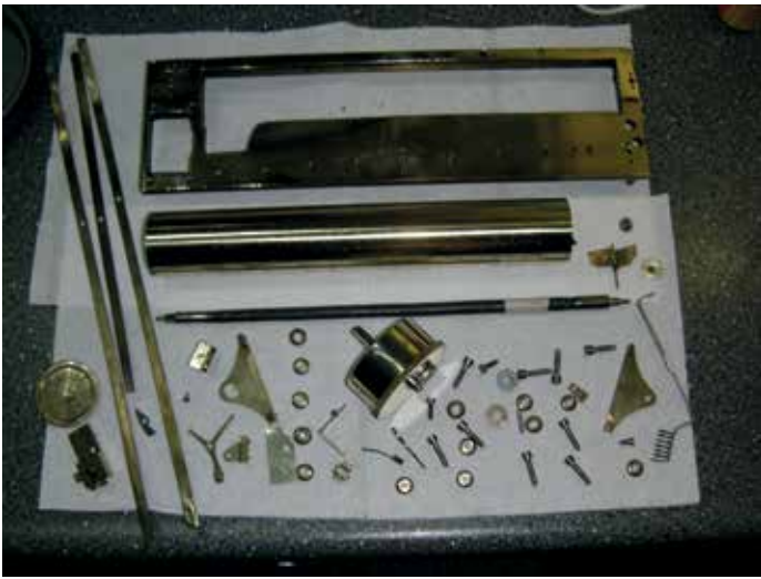
Some serious dismantling of a cylinder box here
