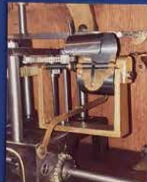
GOVERNOR - STOP ARM - WINDING RATCHET All now repaired. There was just one wing of the air brake hanging on but damaged, and the other wing torn completely off. The air brake and spring were both over tight on the endless worm shaft causing a very hard sudden stop. And all teeth worn on the winding ratchet. See other photo. Friction springs and new air brake wings have been fitted. The worm stop lug replaced and the ratchet repaired.
