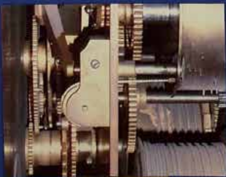
Chain driven time select mechanism. The linkage behind the dial still to be seen.
