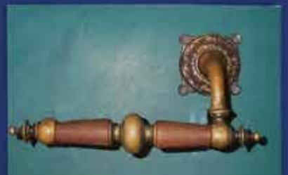
Bin door handle. This job has been in progress for a while. My guess is the bin has been overloaded with the museum's collection of discs. The disc holder collapsed and the door and discs hit the floor. This broke the handle. I had an offer of a new arm and escutcheon to be made by lost wax casting from the originals we still had. For free! It helps to have friends linked to the Industrial Museum! Work is now underway fitting the castings for re-assembly.
