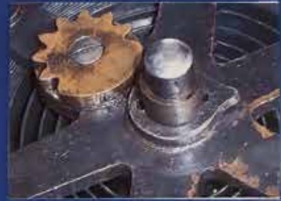
Oops! No driving pin for the stop work finger. The ends of the pin sheared off and missing. This damage could have been done a long time ago.
