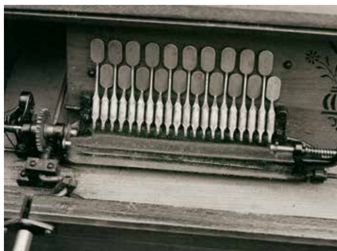
Fig 9: With the cob removed on the Cabinet, it is clear to see how basic the line of keys is when compared to the keyframe of the Grand.
