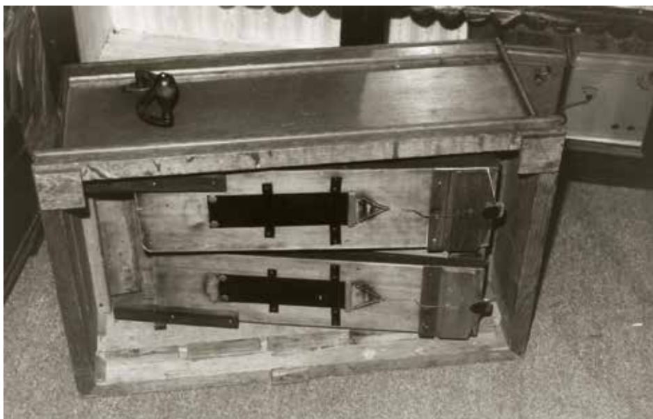
Fig 10: On the Grand, the two exhausters showing the flaps valves before I replaced them and cured the lack of volume.
