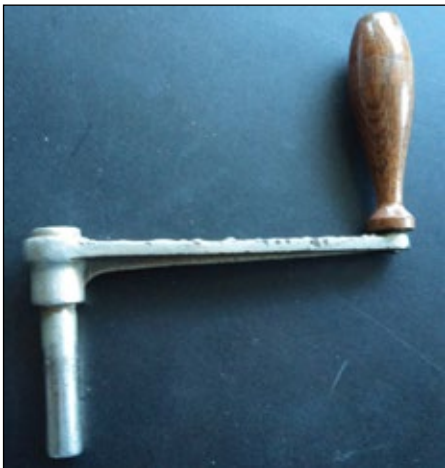
The top photo shows the fancy cast pattern on an original crank handle while the lower photo shows a side view. These images were used to make drawings so new crank handles could be cast.
