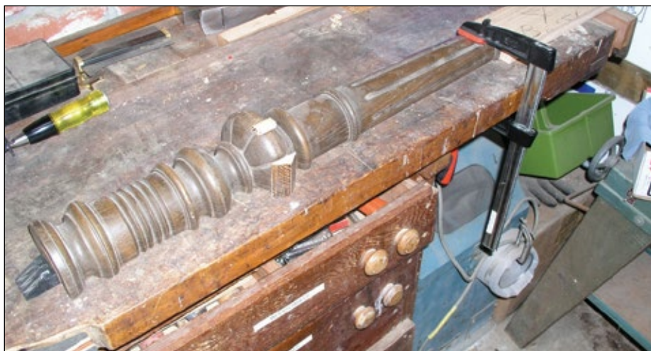
Chunks of wood are fitted to the door columns in preparation for finish carving.
