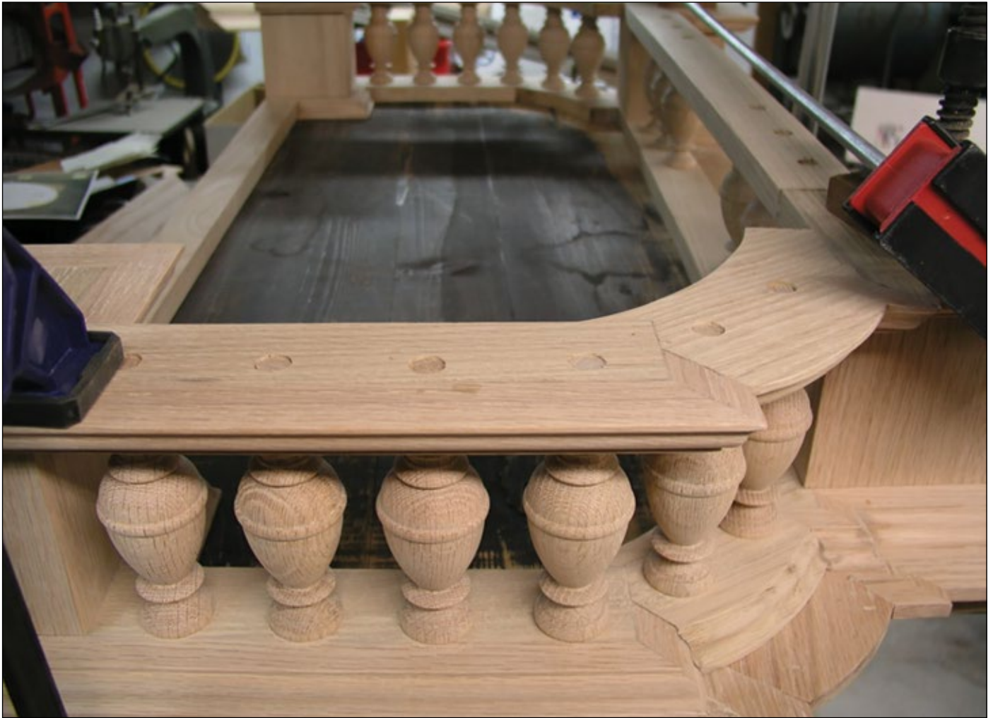
The top gallery including spindles, corner blocks, and top molding is left to dry.
