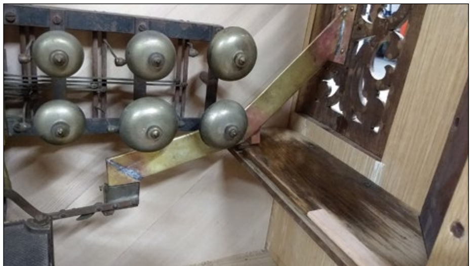
The new coin tube installed just under the bell assembly.
