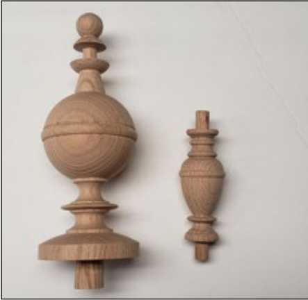
Finished CNC turned finial and spool ready to be stained and installed.
