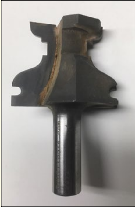
A closeup showing the lower door mold-ing cutter.
