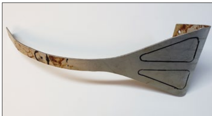
A mockup of the disc support bracket was made out of aluminum so it could be bent into the needed shape.
