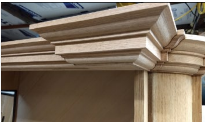
An all new solid oak molding made for the upper part of the top section (below the gallery). Note the elaborate corner details.
