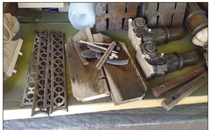
Repaired parts sanded, carved and ready for the refinisher.
