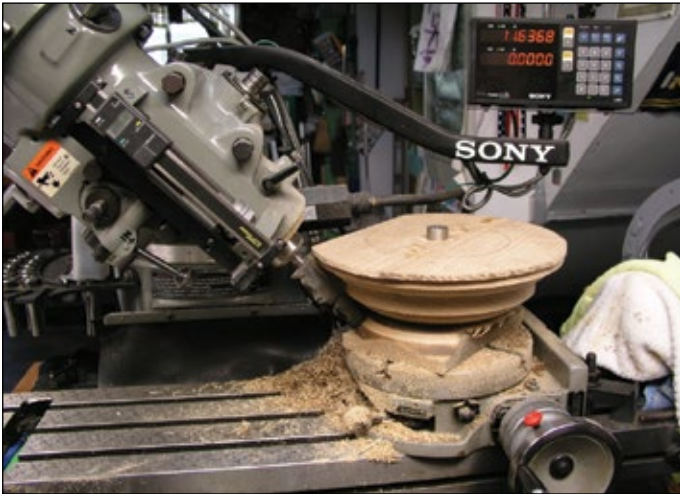
Making the round corner moldings for the upper top section.
