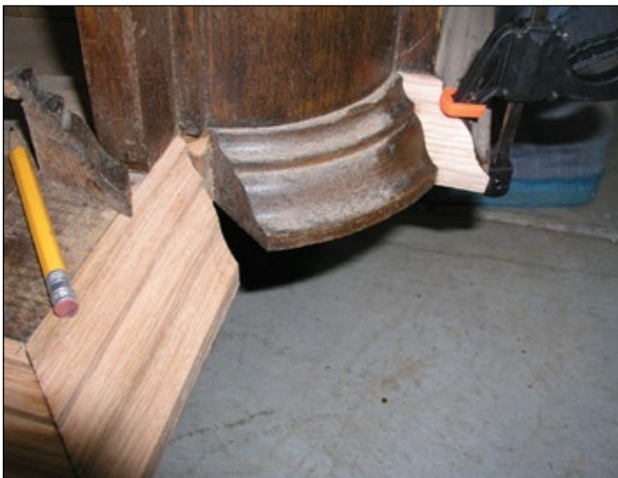
The bottom of the case showing missing moldings being fitted in. Note the double miters.
