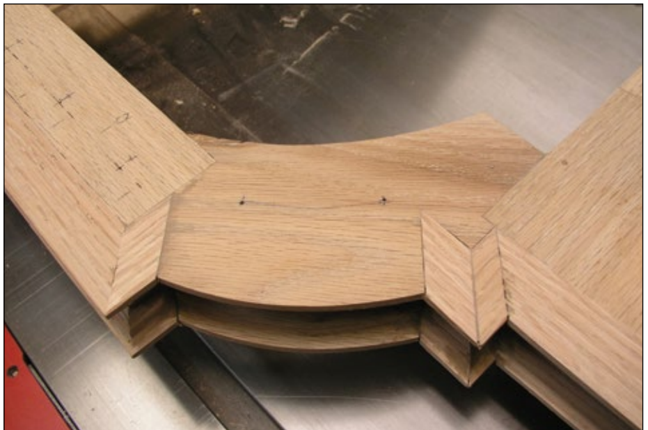
The top gallery features a complex molding configuration. Careful attention was paid to grain directions
