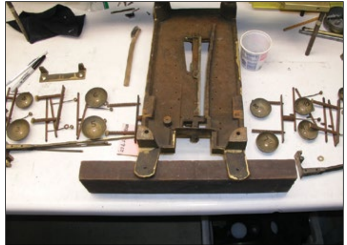
The bell assembly was completely disassembled, and great care was taken to identify where all the parts were located so that they could be put back the same way.
