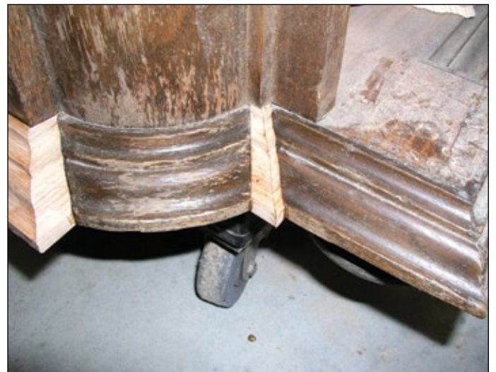
The bottom of the case showing missing moldings being fitted in. Note the double miters.
