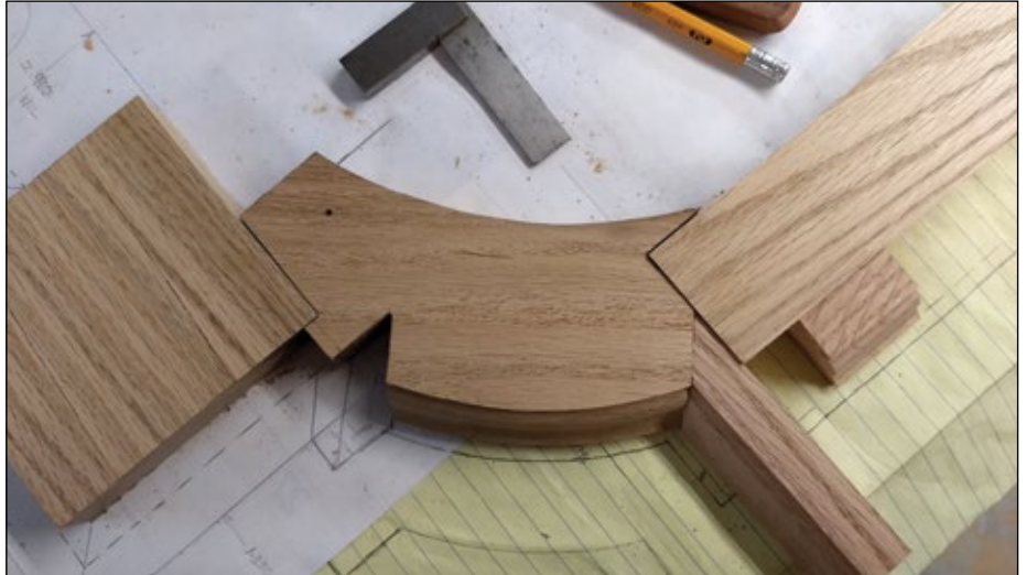
The top Gallery was laid out on paper to scale and the needed pieces were made to fit the layout.
