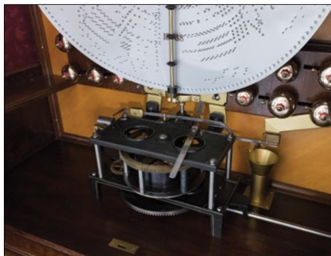
The motor installed and ready to play a disc.
