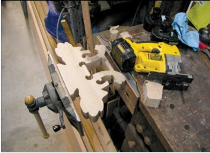
The top crest cut is cut out and made ready for carving.
