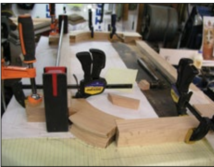
Custom made parts for the top gallery are glued together before installation.
