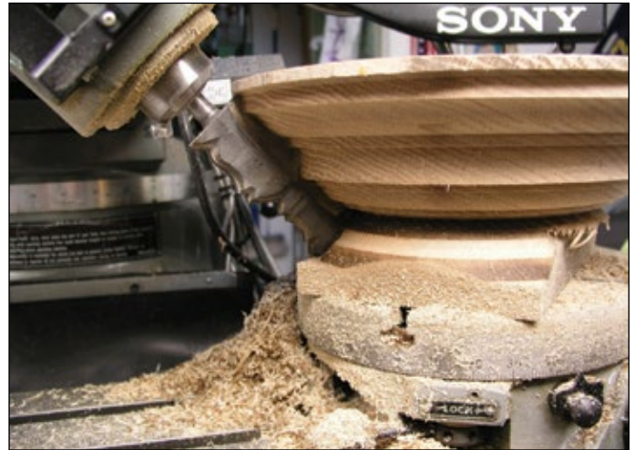
A close up of routing operation for round corner moldings.
