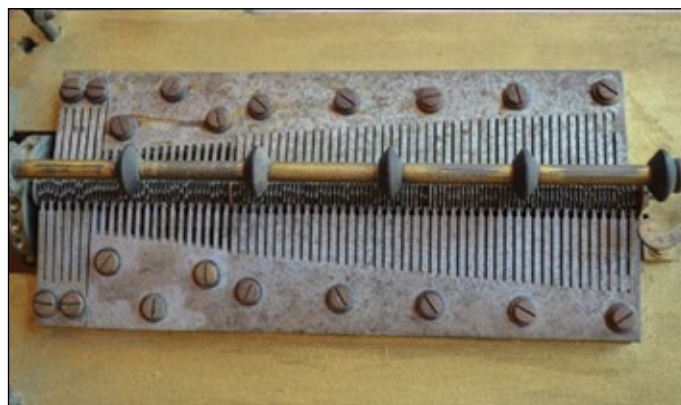
The comb and bedplate as received. Fortunately, the combs had very little wear and only light surface rust.
