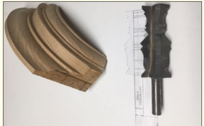
An example of the CAD drawing that is compared to the molding before a custom router bit is created.
