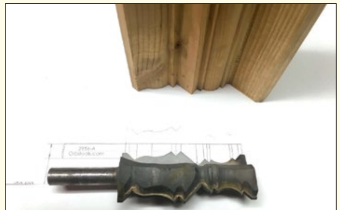
CAD drawings and cutter for moldings shown with the resulting product.
