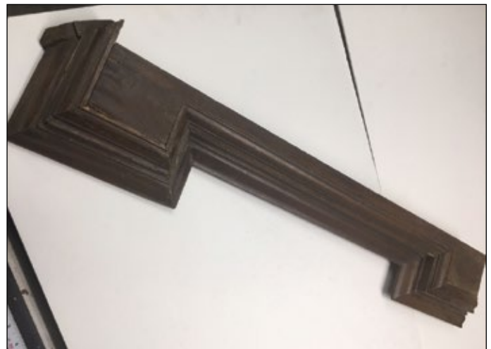
The top section molding as received with pieces missing and veneer coming loose. The molding is shown upside down. A completely new molding was created in solid oak.
