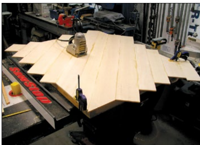
Remaining Sitka Spruce boards are laid into the diagonal pattern and trimmed to the correct size.
