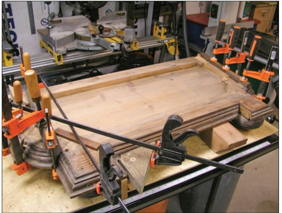
The bottom of the lower-case section being glued back together.
