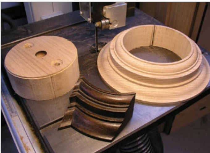
Finished round molding with center section cut out and ready for cutting segments needed to make other pieces like the one shown.
