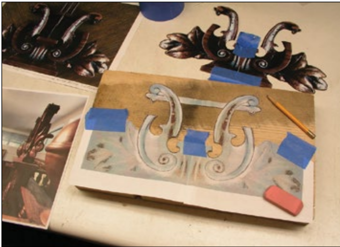
Enlarged pictures were used to get the proper dimensions for the top crest carving.
