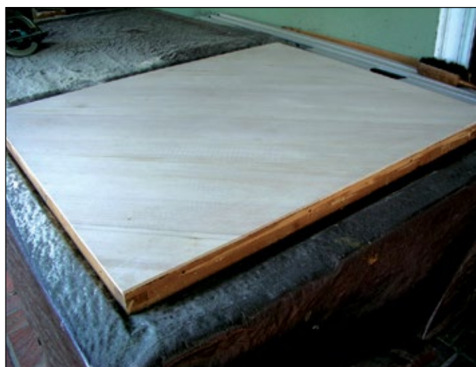
The finished soundboard prior to installation.
