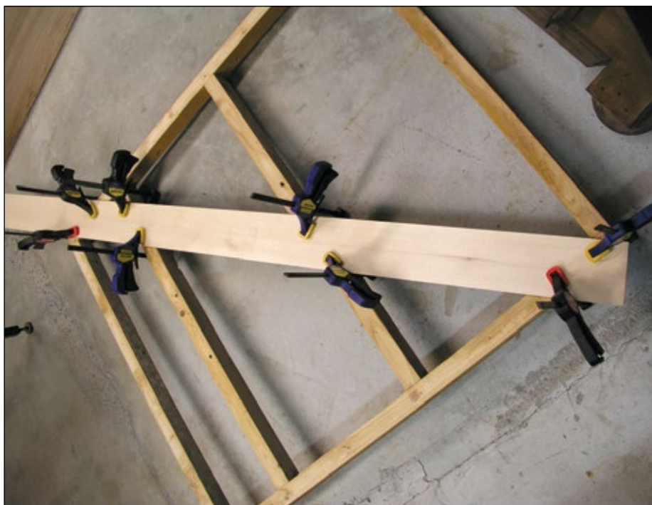
Frame for the new soundboard is laid out and center board glued in.
