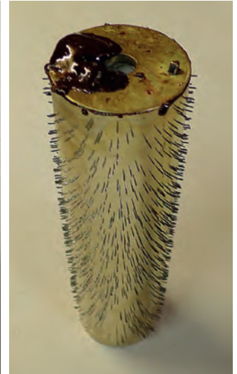
fig 10: Drive hole endcap pushed into place.
