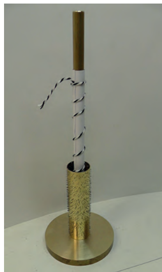
fig 7: Cylinder ready to be filled with cement.
