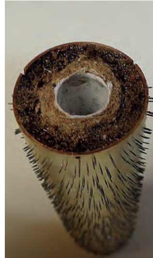
fig 9: Open end of cylinder cleaned and ready for drive hole endcap.
