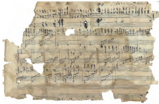
fig 4: Paper saved from the 31.5 cm cylinder of Rzebitschek nr.19082, on the left side remnants of tabs cut into it abut against the endcap.
