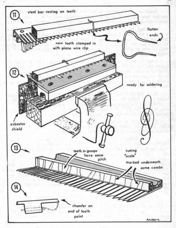
Remember it is better to fit too large a lead than too small as you can tune the tooth up in pitch by removing lead with a pair of fine side cutters. Peg the damper wire into its little hole if applicable.
