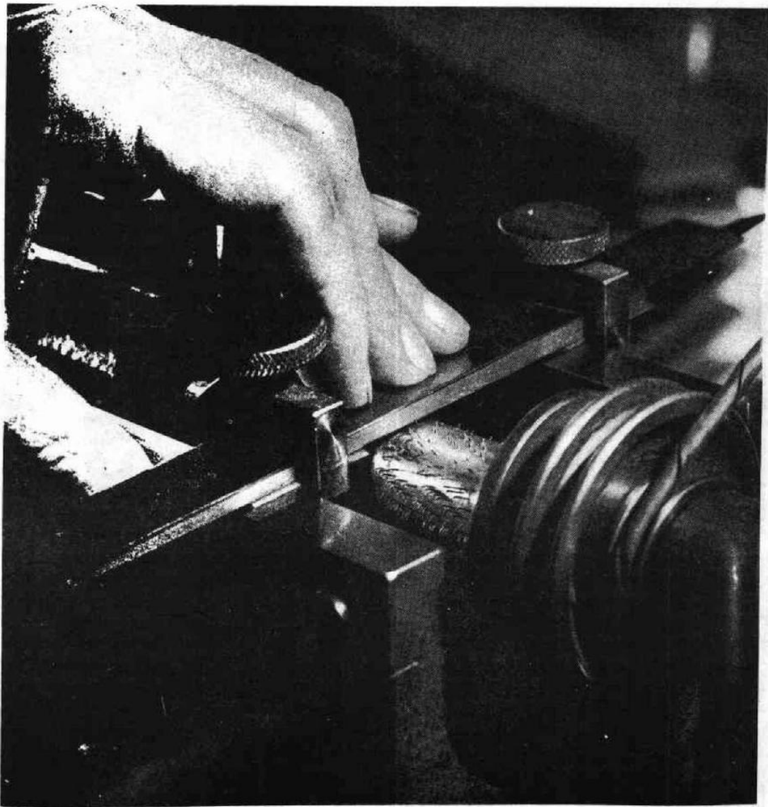
4. The trimming consists in seeing that all the pins are exactly the same length.
