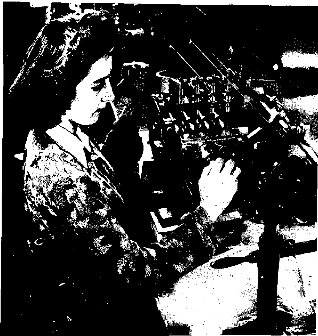
2. Pricking the cylinder, that is perforating the holes in which the pins will be placed, is done by means of clever machinery, according to the seen near the right hand.
