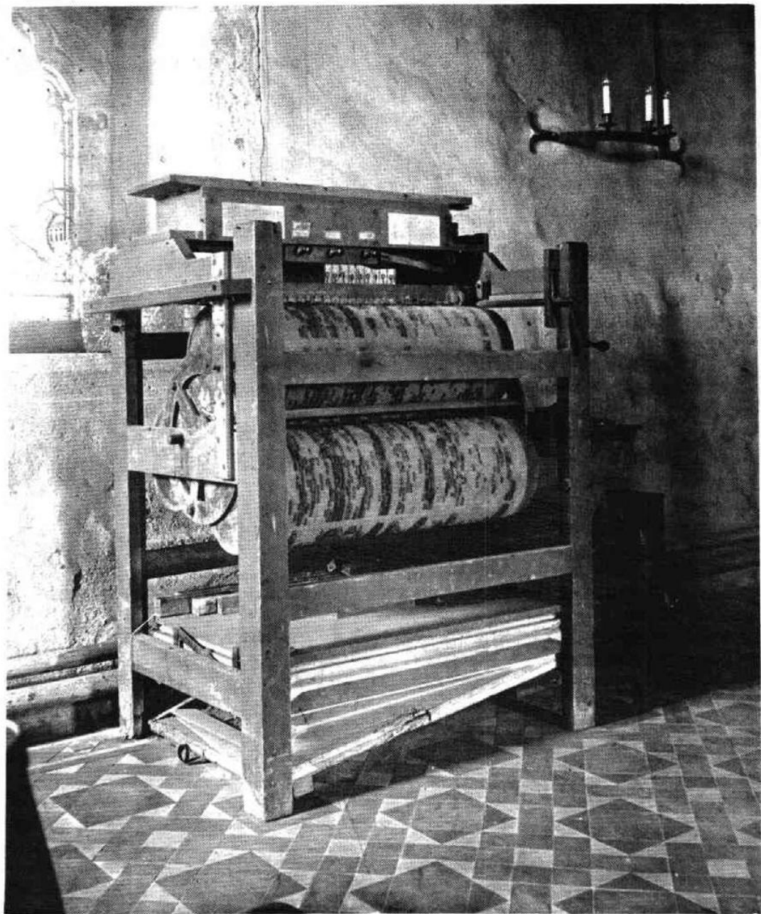
Piddinghoe Church in Sussex contains these remains of a large barrel organ. Three barrels can be seen mounted in a rotating, indexing frame and the soundboard, now without pipes, forms the top of the instrument which no longer has a case. Langwill & Boston state that the organ has three stops and 28 notes. There were ten tunes to each barrel. It is said to have been restored in 1790 which date seems extremely early for an organ of this type. The maker is unknown.
