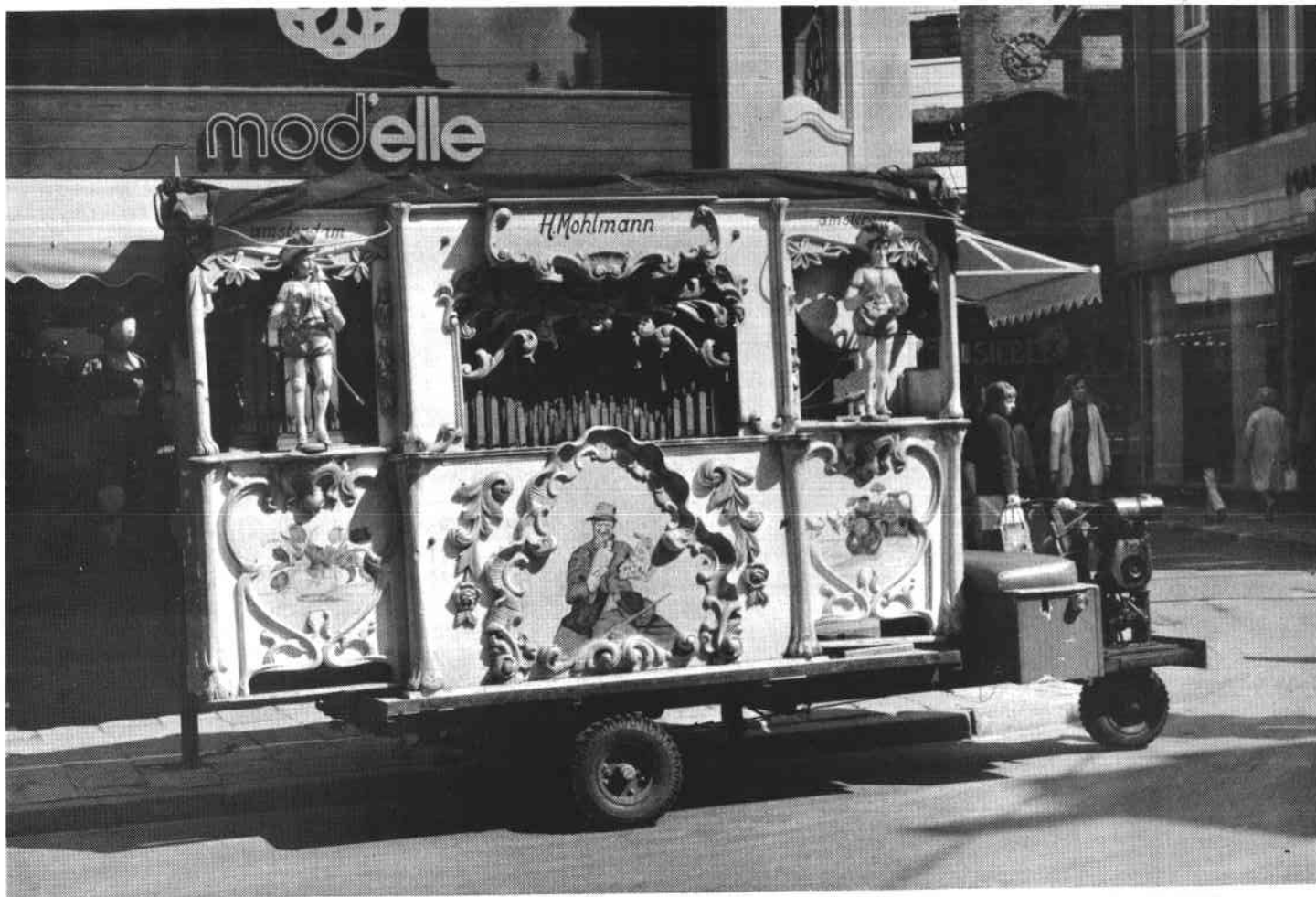
"De Blauwe Trommel". Note the three-wheeled chassis powered by a 7 h.p. JLO engine driving the front wheel. The organ, of course, is hand-turned.
