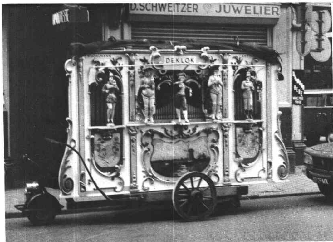
"De Klok", the trailer being fitted with handles for pushing, and a front-wheel motor for driving. Details of the organ and its team are also shown at the top of page 363, the upper pictures on page 365 and the lower one on page 366
