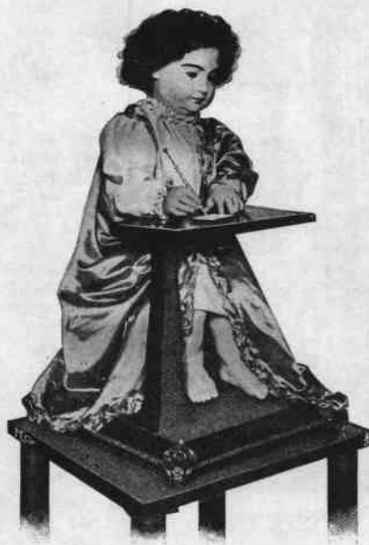
"THE WRITER," A MECHANICAL FIGURE MADE BY JACQUES DROZ IN 1760, WHICH DIPPED ITS PEN IN THE INKPOT, AND COPIED SENTENCES CONTAINING AS MANY AS FORTY LETTERS.
