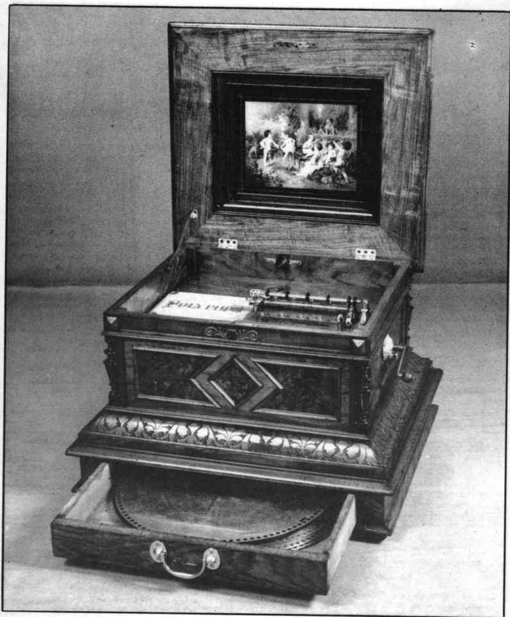
From Member Keith Harding comes this illustration of a fine example of the early-style 15½in. Polyphon with drawer in the base for extra discs. This style entered production about 1895. The two combs together comprise 156 teeth.
