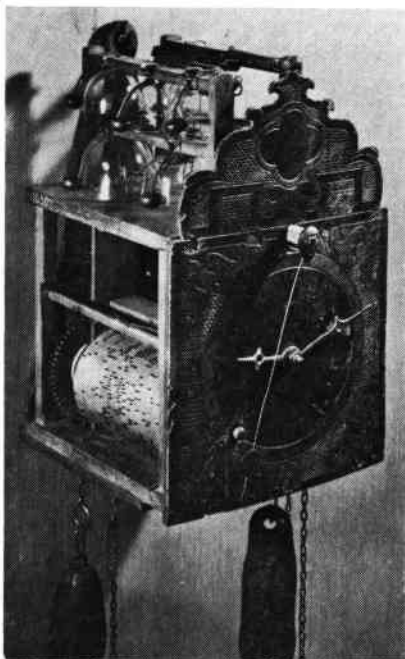
Dating from the second half of the 18th century, this carillon clock by the Prague watchmaker Josef Uhl plays on 12 glass bells. Characteristic of the period is the cow-tail pendulum in front of the clock. From the collection of the National Technical Museum in Prague.
