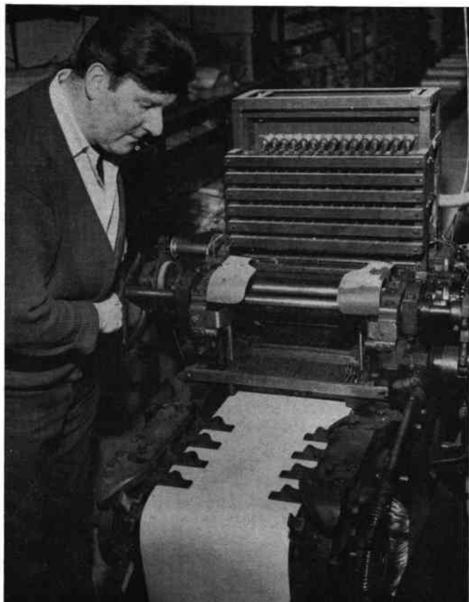
Gordon Iles as he is today. Using original Aeolian Company roll-perforators, he works at his Ramsgate, Kent, home making piano rolls under the Artona label. His company, Artona Music Rolls, has been in operation for many years as a latter-day cottage industry.
