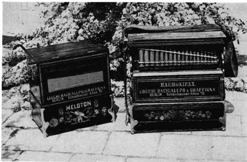
Two of Leon Warnies' original "belly organs". Both date from the 1870's, that on the left being a Meloton reed barrel organ and that on the right a Harmonipan flute and piccolo barrel organ. Both were made by Cocchi, Bacigolupo and Graffigna in Berlin (see the picture on page 239). Both organs are preserved in the Nationaal Museum van Speeldoos tot Pierement, Utrecht, by whose permission this picture was specially taken.
