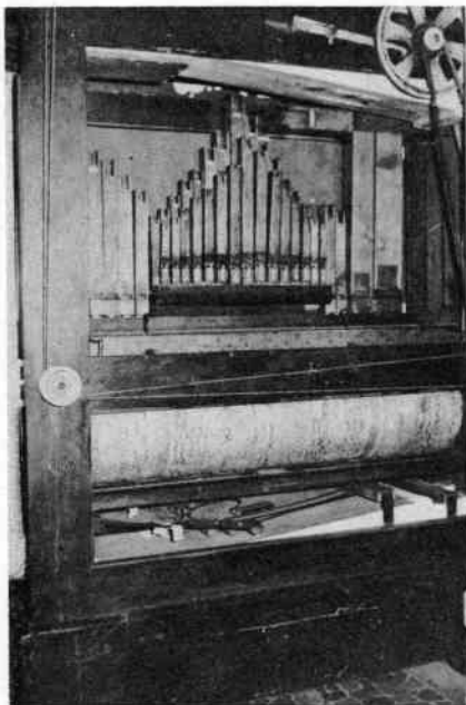
Bob Finbow's 62-key Gavioli trumpet barrel organ shown during restoration. The rear of the organ is seen here along with the feeders and reservoir, the barrel, some of the pipework, and at the top the extra feeder fitted by Bob Minney. At the top right is part of the drive via an electric motor. The cord running around the pulley at centre left turns one of the spiral columns at the front of the instrument. On the right is a view of the organ as purchased by Mr Tyler. The three sections of the organ are here clearly visible: the original ventral organ and the two later drum wing additions.
