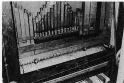
Above is a detail of some of the pipework and the barrel. To the right is the present drive to the crankshaft via electric motor and pulleys. To allow for the not uncommon distortion of the barrel the keyframes ride on the barrel by means of the two adjustable rollers clearly seen here. Note that the wooden pipework in the centre — the string-toned pipes — have the Gavioli frein harmonique fitted to the mouths. On the right is a close-up of the centre section of the organ. This is the total extent of the instrument when originally built.
