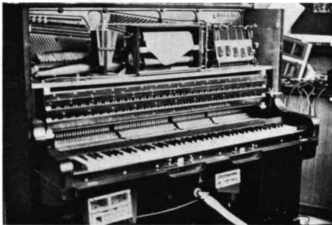
Above left: The Mörs Berlin-made piano which Professor F G Heath rebuilt for computer-encoded magnetic tape playing. The vacuum chests have Perspex fronts to reveal detail of action. Above right: The aluminium rod machined to fit between the tracker bar and the pneumatic stack to take 88 coils and solenoids in the 1974 experiment. The system was not considered reliable and was discontinued. Latest developments involve the use of the system shown in Fig 3.
