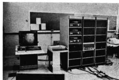
Fig. 5. The computer system by use of which the music is encoded from keyboard (or roll) onto tape.
