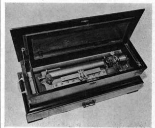
Mahogany cased MERMOD FRERES musical box, the 37cms cylinder playing six airs on single comb, with tune indicator, zither attachment and Mermod Parachute check. Large spring barrel having outside ratchet and the governor playing slow or fast.
