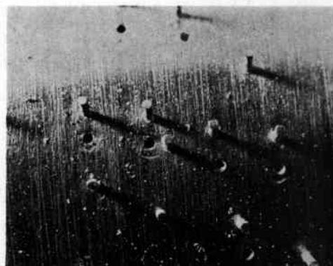
This photo shows the incorrectly marked holes in the cylinder of the movement shown above, and also the new pins.
