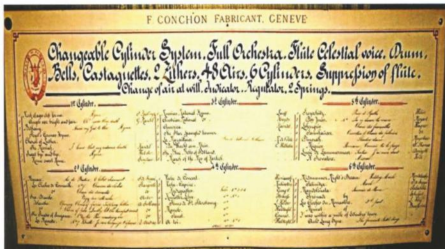
499. Conchon 8496: On a large orchestral box typical of Conchon, the description of its features reads like a short story. The Serial No. is at bottom center along with cylinder length and diameter in pouces and lignes (18 pouces = 19" (48.26 cms); 32 lignes = 2.84" (7.21 cms)). The left music comb has 49 teeth, and the right 46 teeth. The massive case amplifies the sound well, the box sounding quite good when played with the lid closed and all extraneous gadgets silenced! Box made around 1889.
