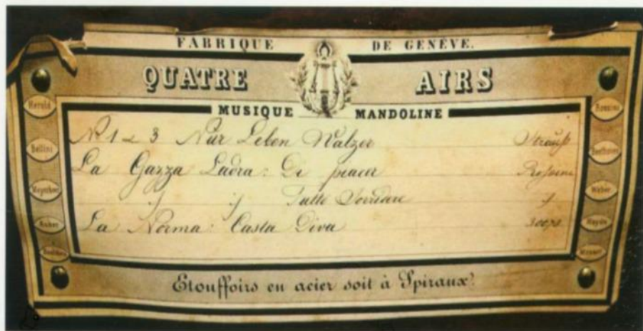
464. Ducommun Girod 30073: The “Musique Mandoline” heading is not an idle boast; a key-wind, super-mandoline instrument with a 13” x 2 1 / 8 ” (33 x 5.4cm) cylinder and a comb with 184 musical teeth. Tune 1, the Nur Leben (Just Live!) Waltz of 1843 is Opus 159 by Johann Strauss Senior. The serial number has displaced Bellini as the composer of Tune 4! Box made about 1854. Redrawing being often necessary with lithograph printing, several versions of this design have been found - see Tune Sheet Nos. 7, 32, 100, 126, 127, 195, 196, 313 & 464; main variations: border shading, redrawn “mask-above-lyre” & composers Herold and Rossini changing sides.
